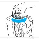
3. Unscrew ring at bottom of tank to remove float stack.
