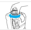
**5.** After cleaning, align arrow on float with tank's notch. Twist ring to lock in place. Ensure alignment to prevent water leakage.
